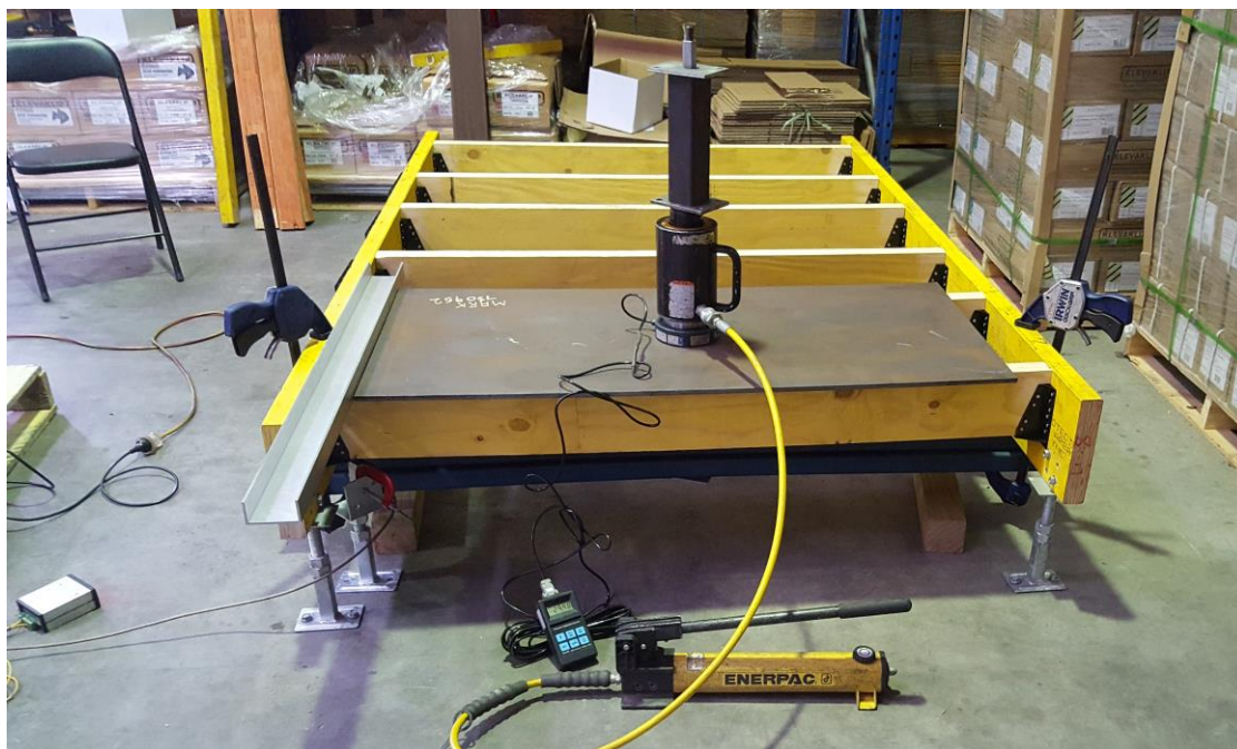
Figure 1: Joist hangers test setup
